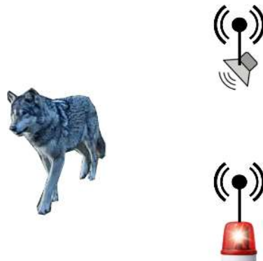
Figure 9.3: The deterrents are activated wirelessly by the system from Figure 9.2 and expel the detected wolf. Exemplary, this figure shows light and sound as two possible deterrents.
