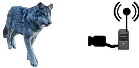
Figure 9.2: The wolf detection works as follows: The detection system uses a camera and a processing unit. Both can be combined in one device. If the model running on the processing unit detects a wolf, it sends a message to the deterrents wirelessly.
