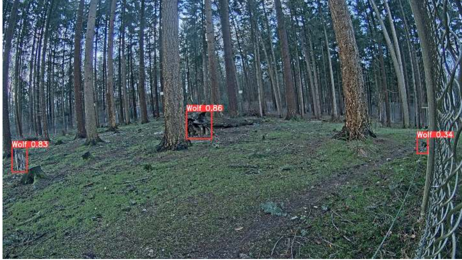
Figure 7.4: Wrong detections of wolves with the base model: The first model detected a tree and an isolator as a wolf.
