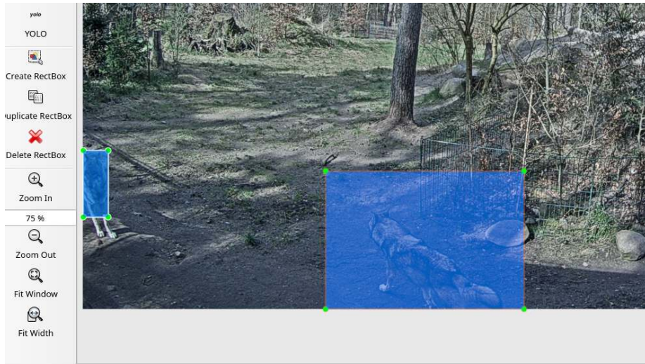
Figure 8.5: The automatically generated training dataset is checked using, for example, LabelImg. The boxes can be fine-tuned to increase the quality of the generated model. The left box could be slightly larger, whereas the right one is too big.
