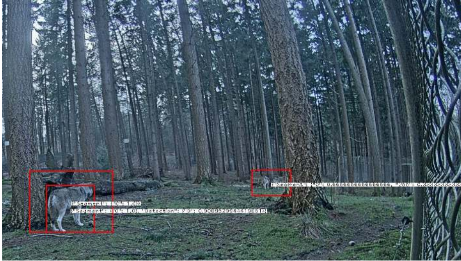
Figure 8.4: Example output from the backmapping module. For the left wolf, there are two segments: One comes from the segmentation and one from the detection. Both have probabilities from Wolf-or-Not . The detector did not recognize the right wolf. Here, only the user-generated probabilities from Wolf-or-Not are available.
