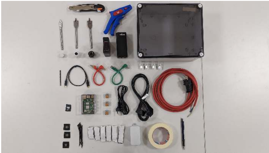
Figure A.2: Overview of the main parts of the camera system according to the Table in Section A.1. Also, some required tools are shown. Not shown: camera, WiFi stick, and ethernet cable for the camera
