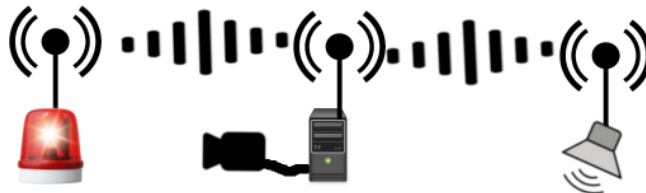
Figure 9.5: After designing the detection and the deterrents, we use LoRa as the communication technology to activate the deterrents and send status messages.
