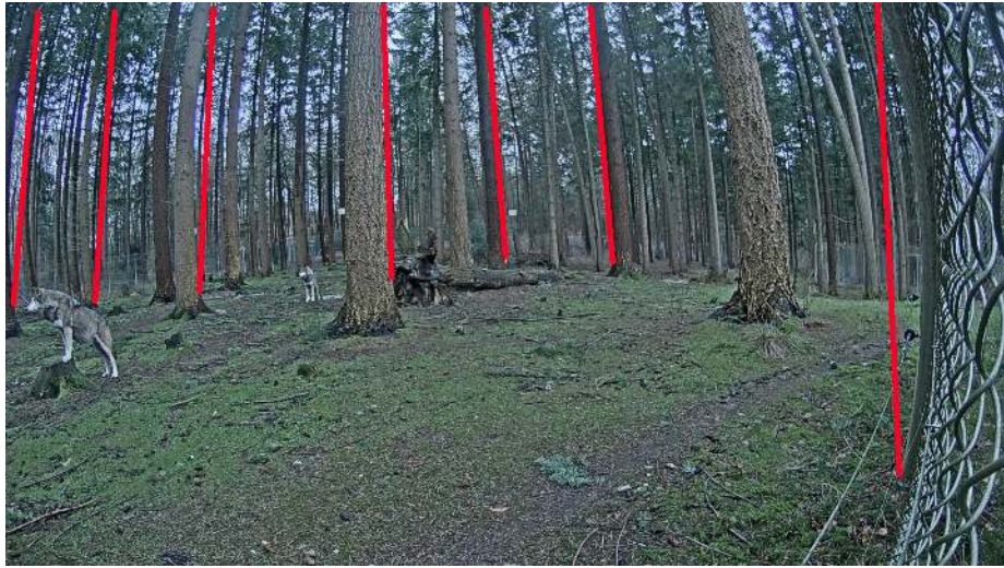
Figure 5.6: The effect of the distortion using a wide-angle camera: The red lines connect two points in the image, which should be straight like the trees or the metal pole at the right side of the photo. Due to the distortion, those look more bent the more they are located at the side of the image.
